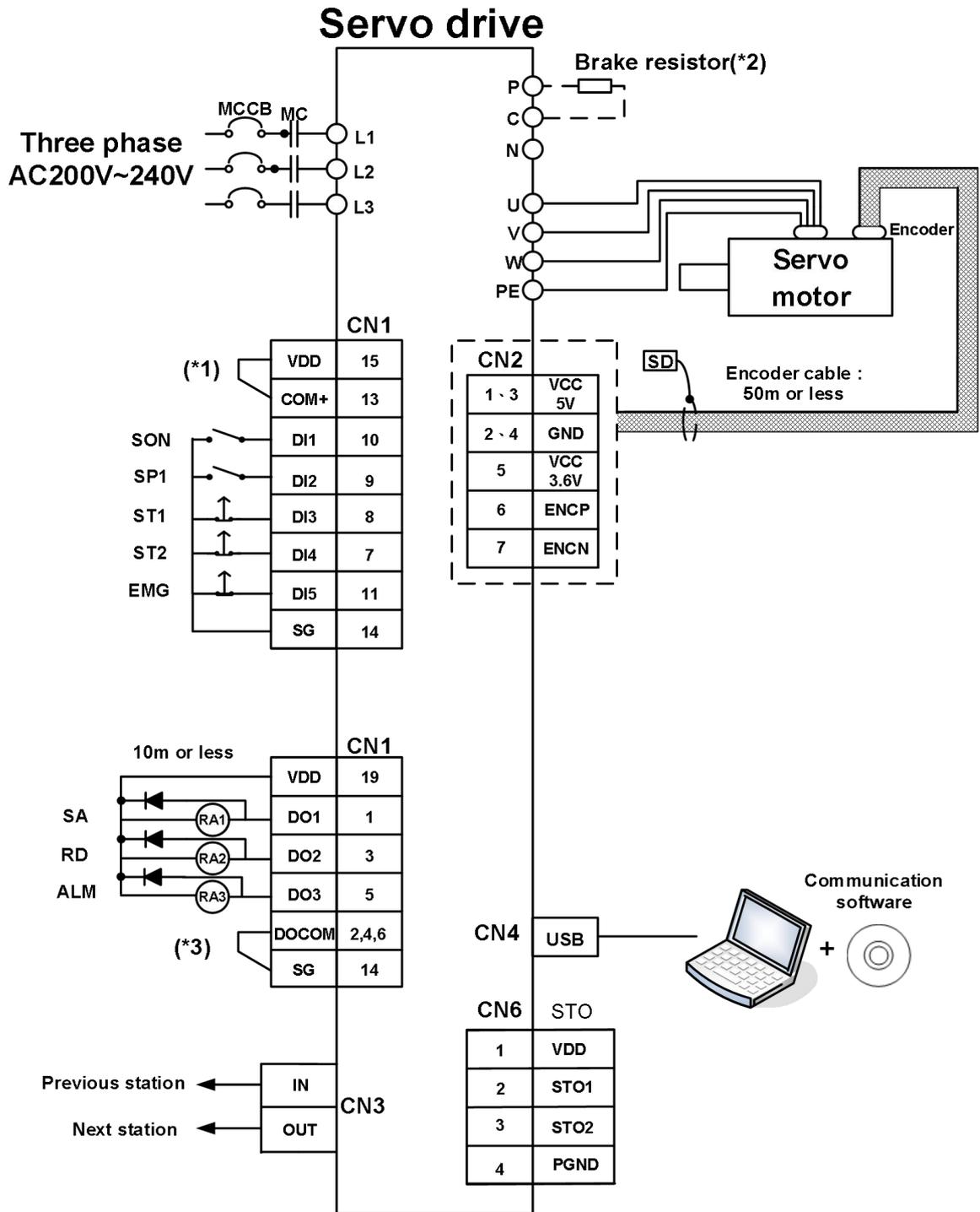
Note1: If an external power supply is used, VDD and COM+ cannot be connected.
