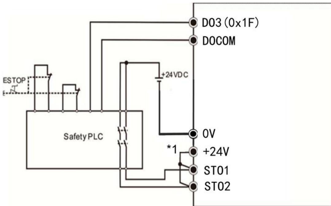
External wiring diagram for STO function
