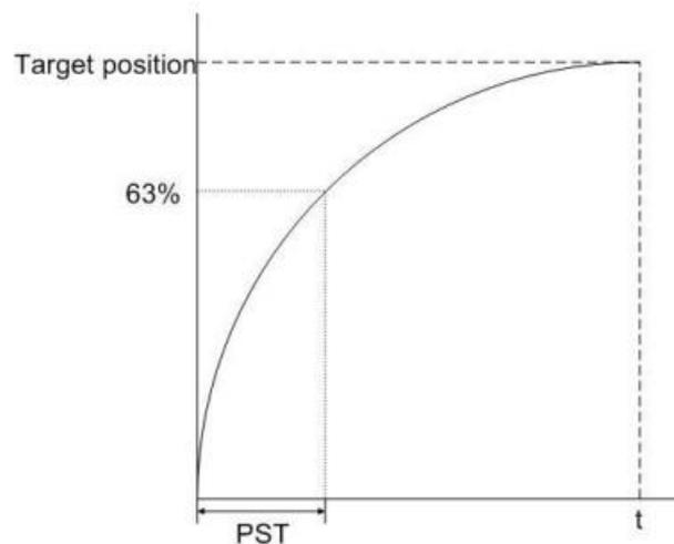
In addition, speed smoothing for acceleration/deceleration can also help the servo motor to run smoother. The speed smoothing parameter for position acceleration/deceleration is as follows:
