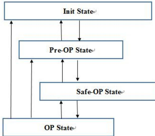
The execution sequence follows the block diagram from top to bottom. The state can be switched from bottom to top as required. If the final state is the same as command, it means switching process is completed.
