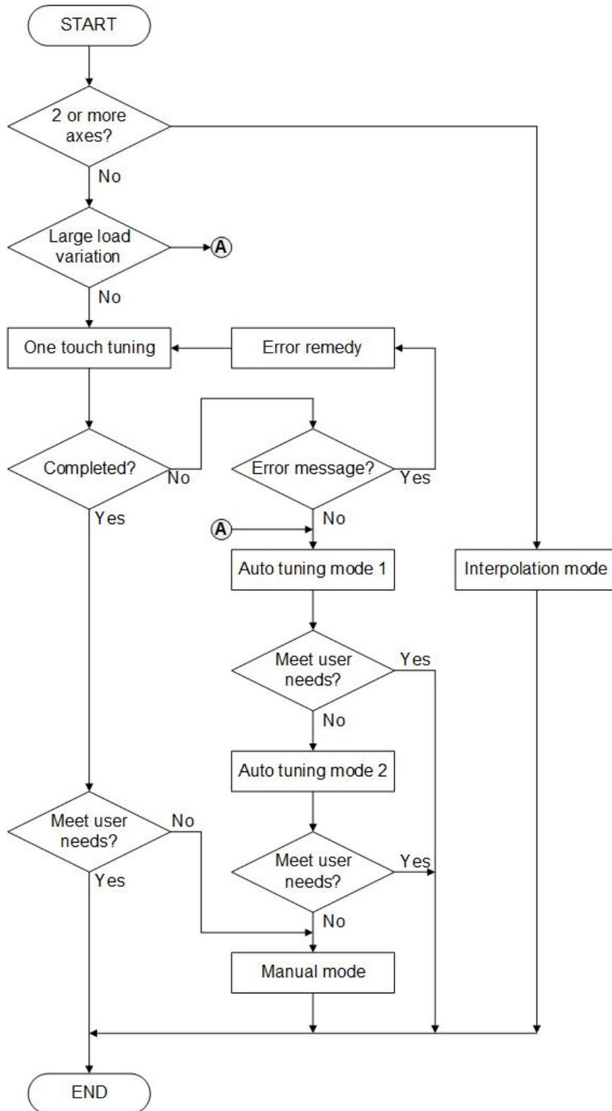
If the servo is being used for the first time, a JOG test is required to confirm no abnormal before using the auto-tuning function. In auto-tuning mode, the servo needs to accelerate/ decelerate for several times, and after the inertia ratio estimation turns to a steady state, the purpose of inertia ratio estimation and bandwidth search can be achieved.
