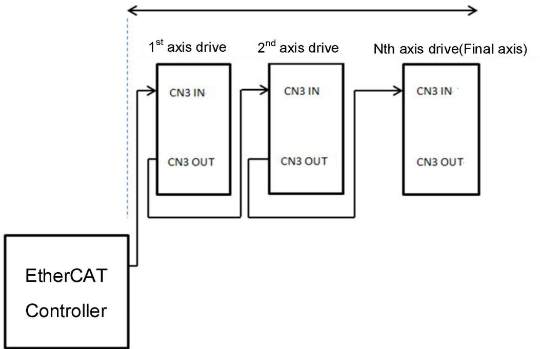
Note 1: The connector for CN3 is an RJ-45 connector.
