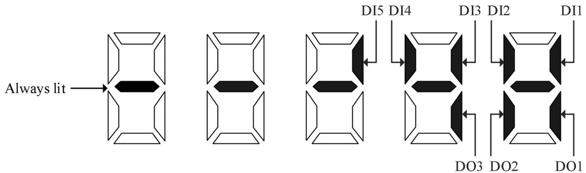
The above figure shows ON/OFF in a 7-segment LED, the upper part is the input signal (DI1~DI5), the lower part is the output signal (DO1~DO3) and OP. When OP is ON, it means that the motor is in the Z-phase position.
