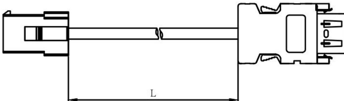
**Medium/high inertia encoder cable:**(for SM3 100W~1KW motor)
