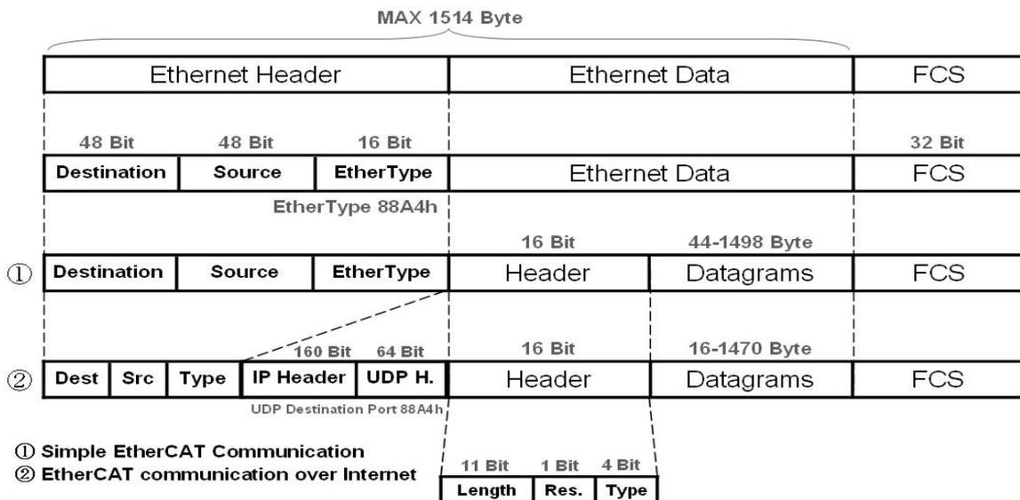
The communication frame includes 3 parts: Ethernet header, Ethernet data and FCS. The Ethernet header contains data source, transmission destination, and the EtherCAT communication mode needs to be selected as EtherType. And Ethernet data content has header and datagrams. The datagrams can set the frame delivery method and check if the read/write action is completed.
