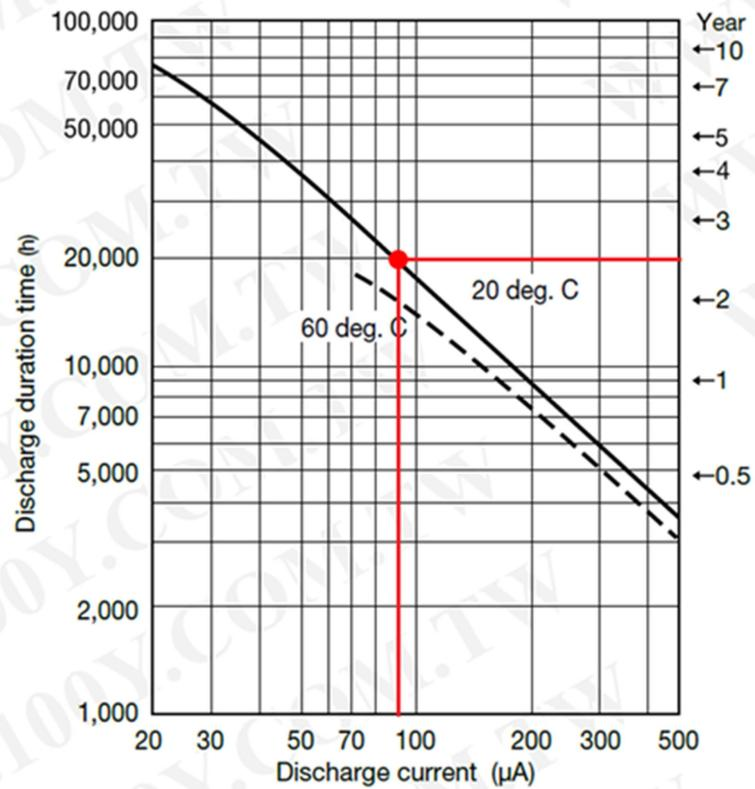
The above graph shows the battery life curve provided by the battery manufacturer. According to the curve shown above, if the consumption current of the absolute encoder is  $90\mu\text{A}$ , the expected battery life is around 20,000hrs, which is equivalent to 2.3 years.
