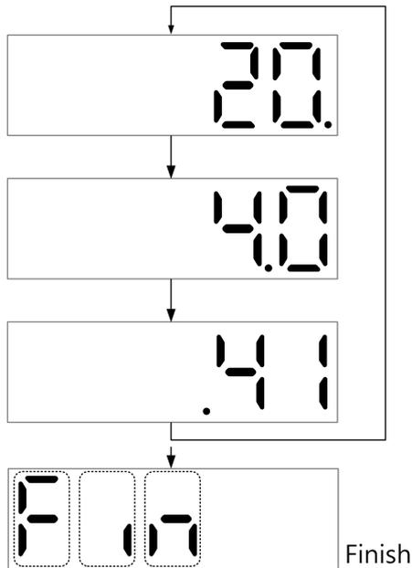
(d) If you want to terminate the process during tuning, press the SET key to stop, the panel display and the troubleshooting process are as follows:
