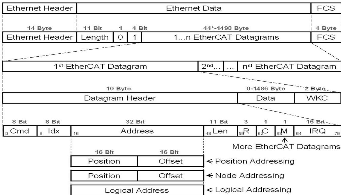
One EtherCAT data frame may contain several datagrams, and the maximum size of an EtherCAT communication frame is 1514 Bytes. The header of datagrams is for the data exchange method selection and the slave address marking, it also reads and writes the EtherCAT internal register's data by determining the slave address.
