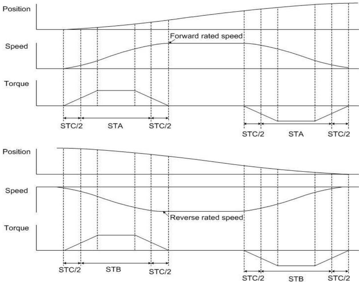
The above figure shows that the acceleration and deceleration times are controlled by (PF49~PF64) when the position command is forward rotation or reverse rotation.
