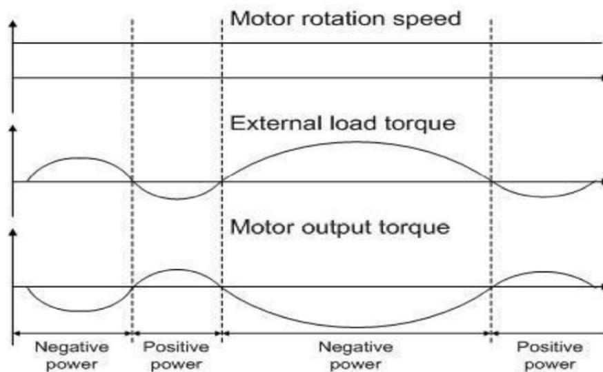
Negative work by external load torque:  $T_L \times \omega$
