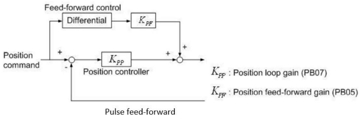
The parameters related to position gain adjustment are listed below:
