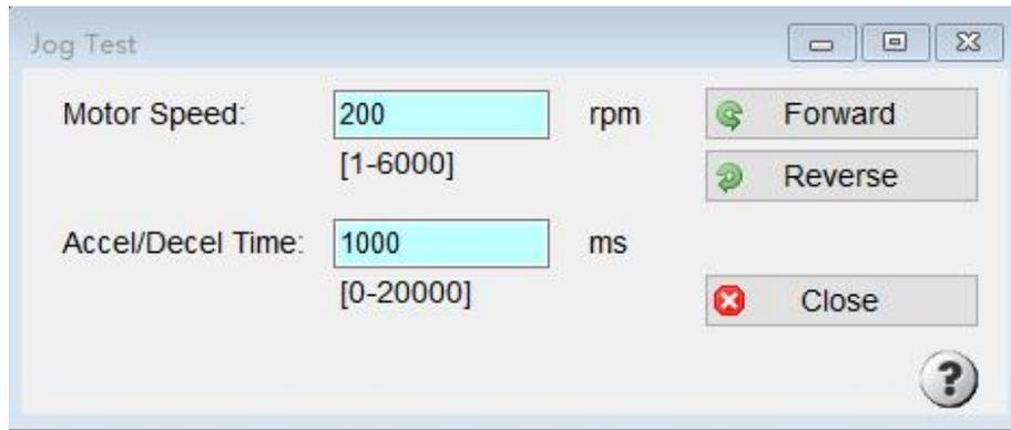
Note: When using the communication software, if the communication cable is disconnected during JOG test, the servo motor will decelerate and stop.
