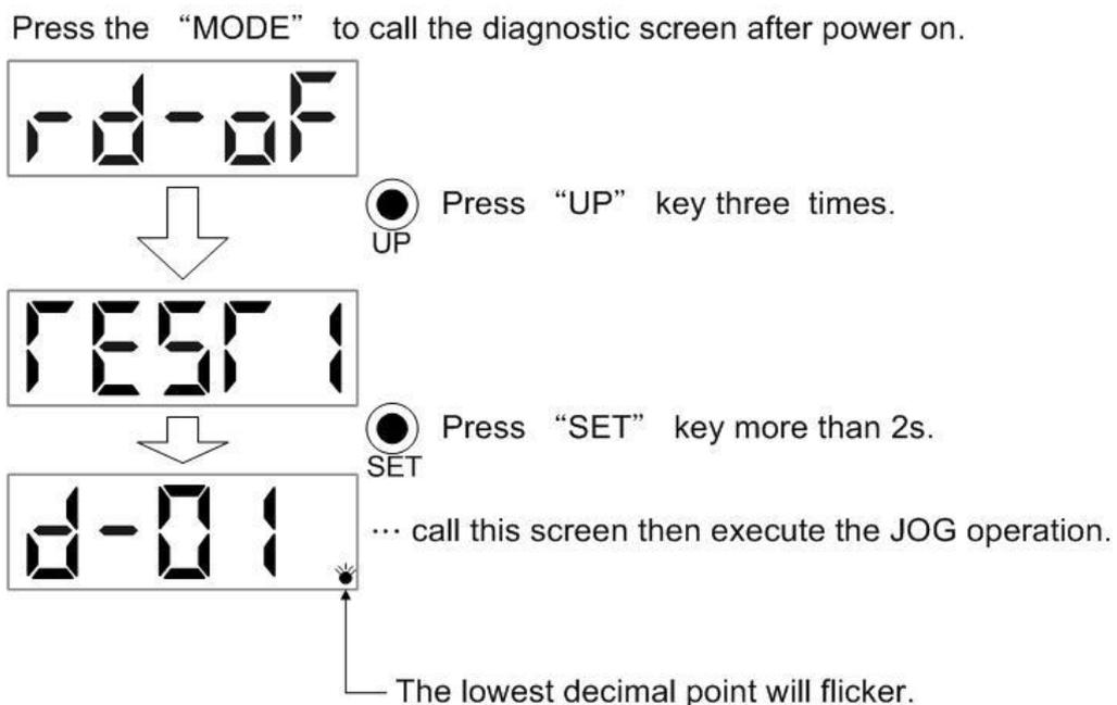
Step 3: Run the JOG test. Press the UP button to run the motor in CCW direction, and press DOWN button to run the motor in CW direction. Release the button to stop. The running speed of JOG test can be modified by PC04.
