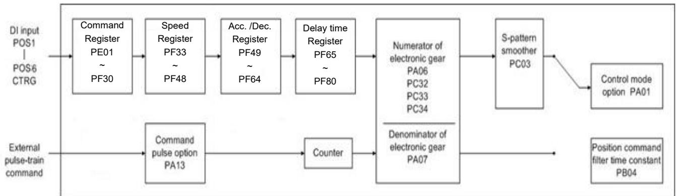
Note: The S-pattern smooth is invalid when the external pulse-train commands are applied.
