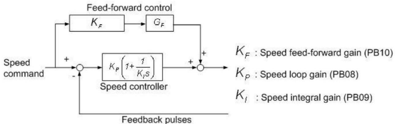
The gain adjustment related parameters in speed control loop are summarized as follows:
