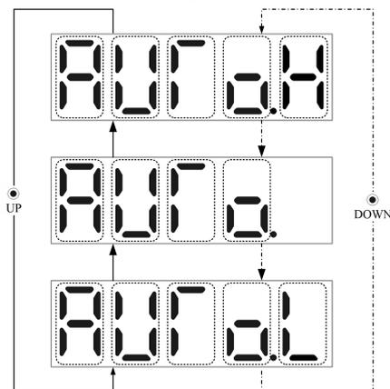
(c) After selecting the response mode and pressing the SET button, One-touch tuning function will be executed and the panel will show the progress.
